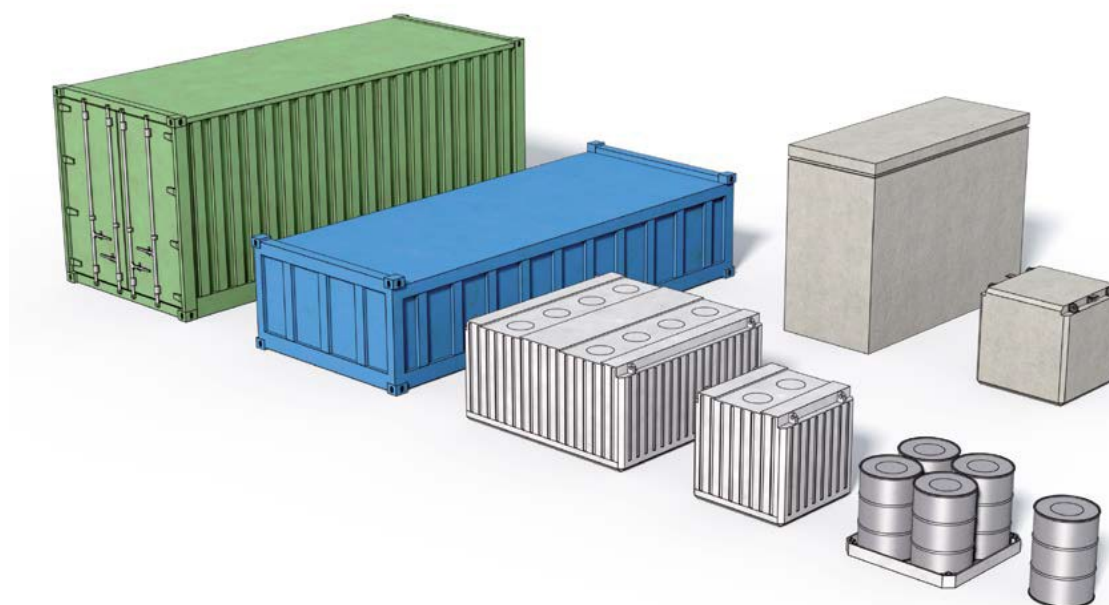
Figure 20: Schematic illustration of waste packaging used or intended to be used in SFR (Sweden).
